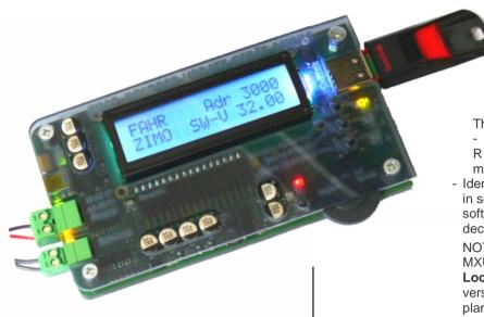
The MXULF - or rather the MXULFA variant, with a screen – is the ZIMO decoder update and sound loading device, and, from software version 0.22, also suitable for driving (ie, with its own control commands, without a computer); from software version0.32, the sound loading via SUSI is also active .
